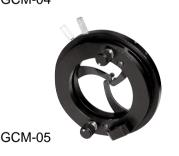
The series GCM-04/05 of Self-Centering Lens Holders offer a reliable and self-centering mechanism for any round optical components. They are very useful when optics of variable diameters must be interchanged frequently and the height of the optical axis must be kept unchanged. Moreover, Adjustable Self-Centering Lens Holders GCM-05 can also be tilted relative to the X or Z axes through  $\pm 4^{\circ}$ .
