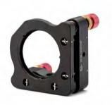
The series of 2D Kinematic Lens/Mirror holders, which adjustment range for single direction is  $\pm 4^{\circ}$ . The thread pair is axially locked, and make the spot more stable during locking process. These holders are more suitable for thinner optics which thickness ≥2mm
