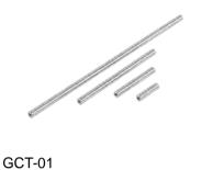
These cage rods are made from stainless steel. The two top ends of the rods are M3 threaded holes with a depth of 6 mm, which can be connected by GCT-540201 screw connector, and can be combined into the length required by the system.
