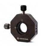
The series of X-Y Lens/Mirror Holder, GCM-083904M, can be used for  $\varphi$  25.4mm optics with maximum thickness 5mm. The adjustment range is  $\pm\,1\text{mm}$ . The holders can be connected to the post GCM-03011 through the bottom M4 thread hole.
